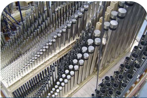
Examples of wood, flute pipes set in their pipe chest. An empty pipe chest is in the foreground: this shows chest holes in which pipes will be set. Photo from Organ Supplies Industries web site.
