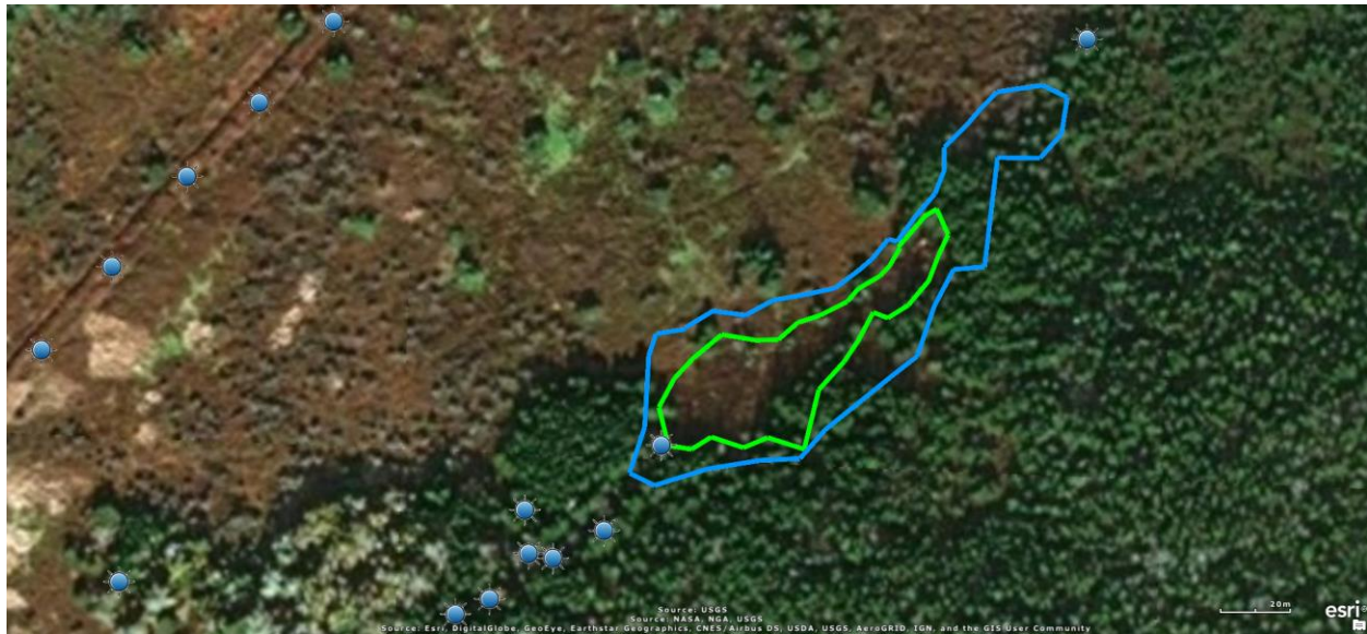
Figure 21: The Big Lily Pond on the southeast ditch had not held water in over 50 years prior to restoration at BMB. Following installation of ditchblocks (blue circles) the open water area recharged to 1950m 2 by May 2017 (green line) and over 4550m 2 by February 2018 (blue line).
