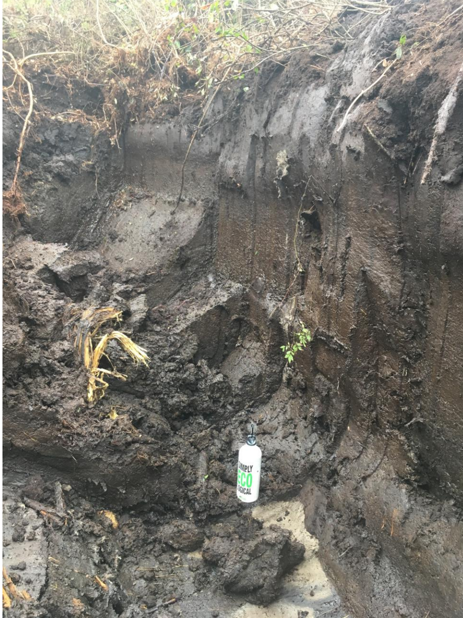
Figure 22: This image of a ditch block borrow pit area in along the northeast ditch shows a peat layer of approximately 0.8m underlain by a light grey mineral soil, and pieces of wood within the peat matrix below approximately 0.5m.
