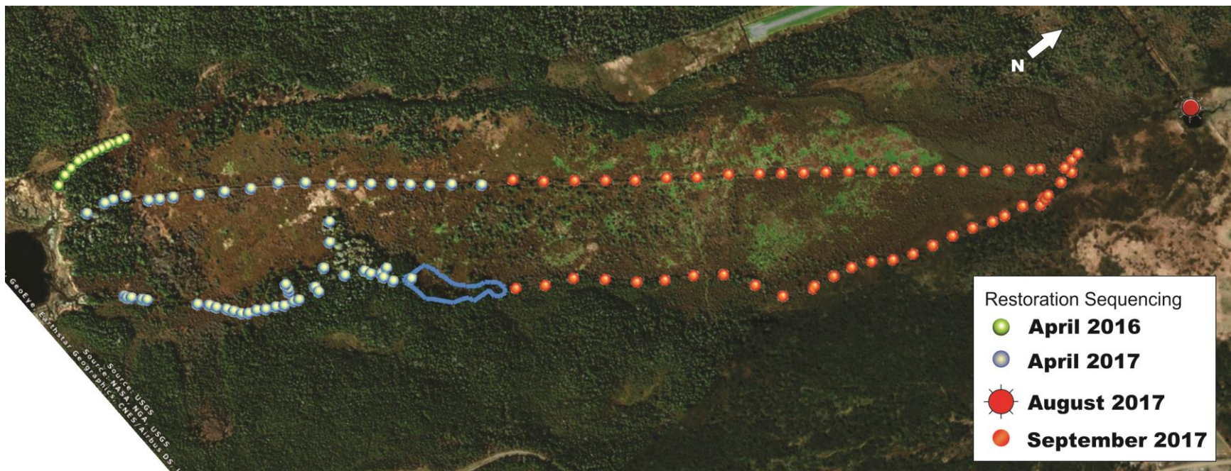
Figure 3: A pictorial representation of ditchblock construction and re-profiling sequencing at Big Meadow Bog. Each dot represents the specific location of a constructed ditchblock. Also shown is the location of Jimmy's Pond restoration site in the extreme north, and the post restoration boundary of the Big Lily Pond (blue line).
