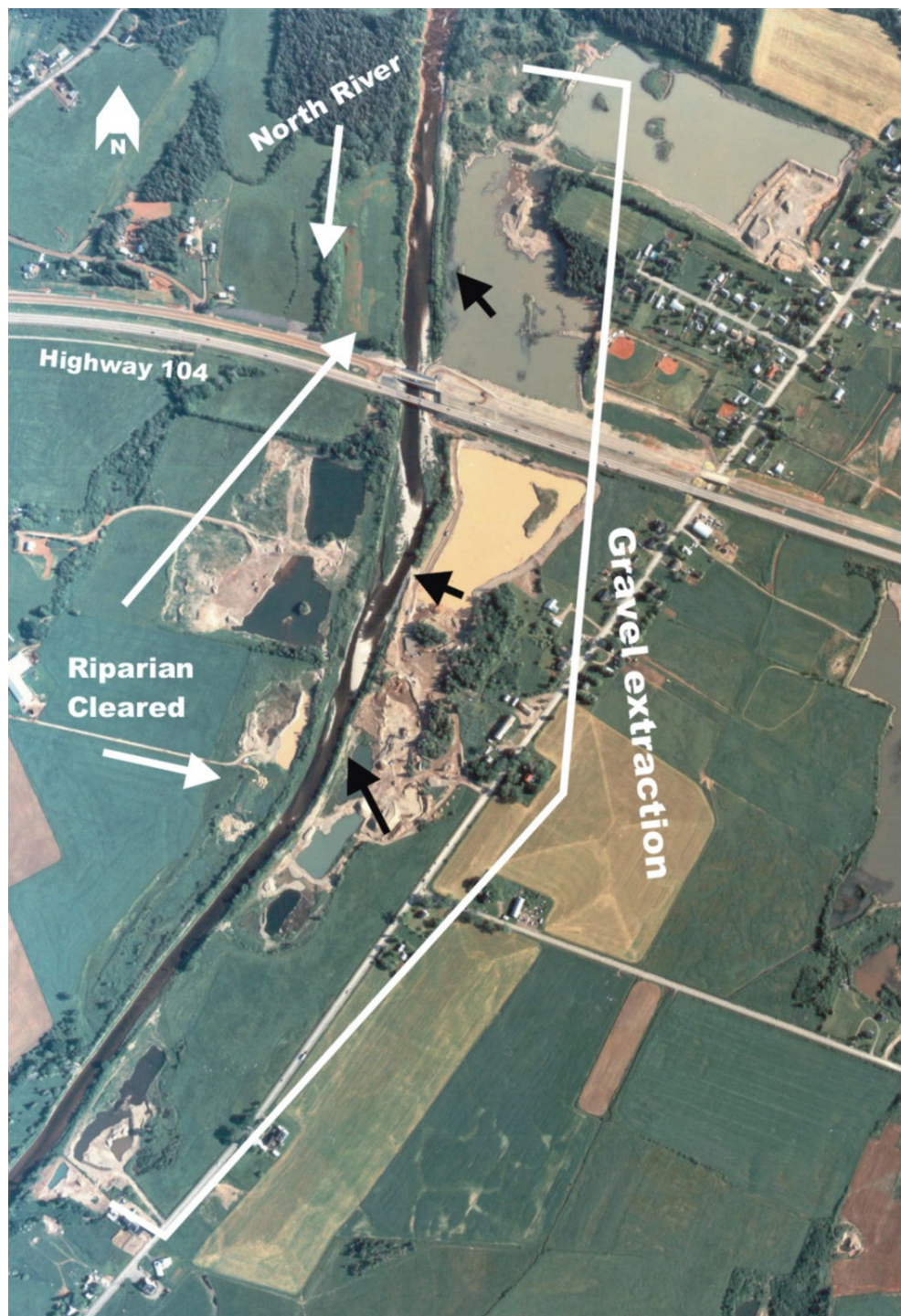
Figure 8: Numerous gravel extraction operations exist immediately adjacent to both sides of the lower North River near Highway 104. Resulting ponds exhibit suspended sediments. Thermal warming and sedimentation may be an issue if these channels drain directly to the river. The North River has been channelized all along this reach (see also Photo 3), and completely lacks habitat diversity.
