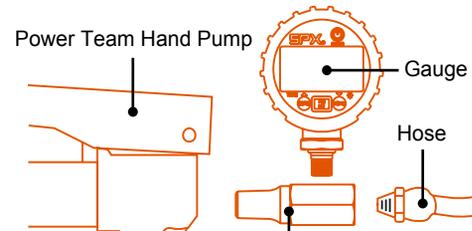
Tee adapter (No. 9670) is used for installing a gauge in line in a hydraulic circuit.
