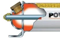
Power Team hand pumps, with the angled fill port, have a built in "relief valve" protection system. This system is designed to protect over-pressurization of the reservoir from sudden back pressure. This system also works as a seal to prevent oil leaks only fill to bottom of threads.
