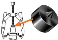
Power Team shaft protectors are designed to protect shaft centers from distortion when extreme pressures are applied with jaw-type pullers or Bi-Directional™ Pullers. Shaft protectors are inserted between the end of the puller screw and the shaft.
