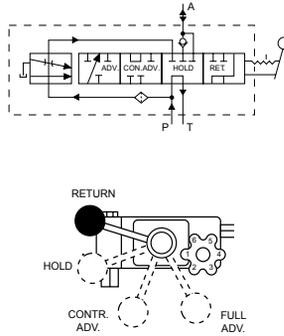
**Applications:** Single-acting cylinders. Primarily for use in testing soil, rock, concrete, asphalt and related engineering materials.
