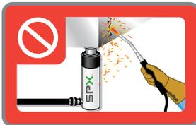
Keep equipment away from excessive temperatures. Do not weld next to unprotected equipment.
