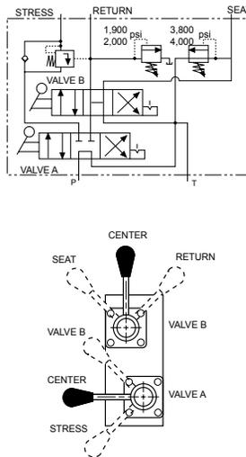
**Applications:** Multi-strand, double-acting stressing jacks with an auxiliary seating cylinder.
