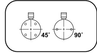
**NOTE:** Base mounting holes are standard on all RD cylinders. \*Orientation of base mounting holes to coupler.
