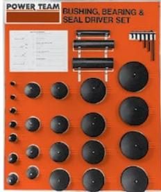
These sets include discs and handles for custom seal driver assembly to provide a pilot (to prevent cocking), a spacer (so force is applied on the proper area) and a driver (for even force dist.). Discs range from 0.50" thru 4.50" diameters in 0.06" increments. Each set includes a handy plastic box with pre-cut tool tray.
