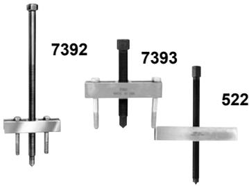
Ideal for pulling many small parts having tapped holes. The 7392 and 7393 may be used with the 1122 pulling attachment to remove bearings, etc. Pullers include two hex head cap screws, 3/8" – 16 NC x 3.00" long. Spread: 1.50" – 4.25". Width of puller block is 4.88". Cap screws are not included with the 522, but any cap screws up to 1/2" diameter may be used. The 522 spread, when used with 1/2" dia. cap screws, is 2"-7 3/4". Width of the 522 puller block is 8.25".
