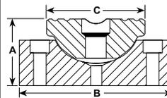
Reduce the effects of off-center loading. Tilts up to 5 degrees. Radial grooves on top of cap reduce load slippage. Notch across face of each cap helps keep loads having a protruding or round shaped centered.
