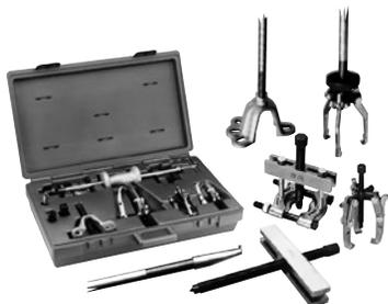
Components can be assembled to create several versatile puller versions. The puller head is turned to securely lock the jaws onto the part being removed. Both a 2-way and 3-way puller head are included, plus three long-reach and three short-reach puller jaws in a plastic storage box. Easily removes gears, bearings and other press-fitted parts.
