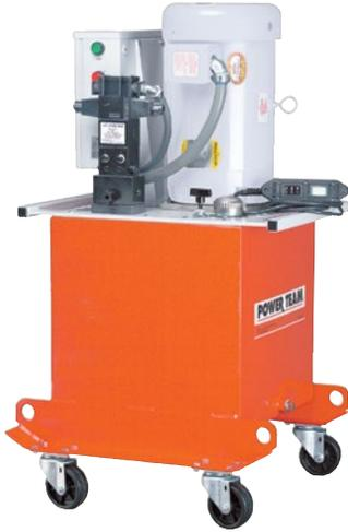
▶ **PE4004S pump and RD3006 cylinder used in a special press which repairs damaged chain links for the shipping industry.**
