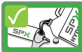
Do not overfill pump reservoirs.
