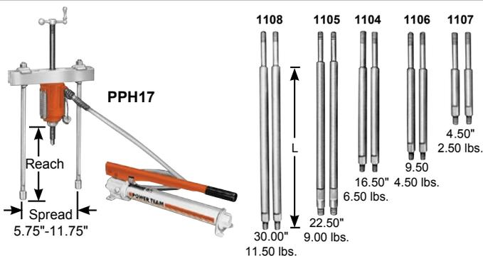
**Leg Ends** – Upper leg ends are threaded 3/4"-16. Lower leg ends are threaded 5/8"-18.00" long
