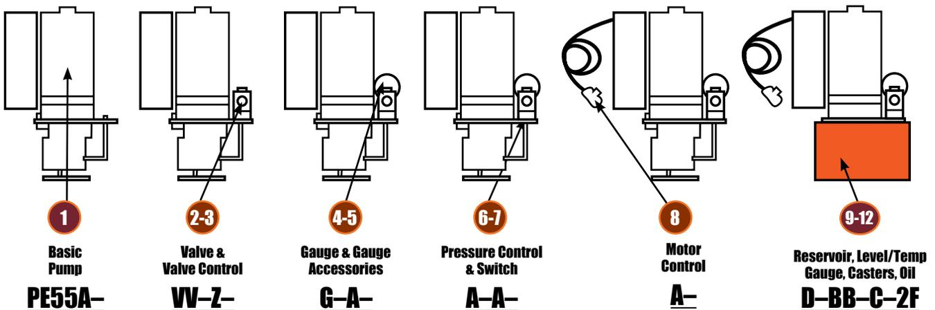
Pump No. PE55A-VV-Z-G-A-A-A-A-D-BB-C-2F is a 10,000 psi two-speed pump with a 115VAC, 50-60Hz, single-phase, 1-1/8 hp, 12,000 rpm motor; a 9512 4-way solenoid valve with a 202778 remote hand control, a 9041
