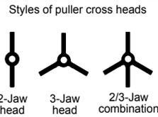
Compare the "reach" and "spread" of the pulling job with that of the pullers listed. The puller selected must have dimensions greater than those of the job.
