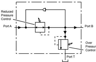
**Application:** Provides complete, independent pressure control to two or more clamping systems operated by a single power source.
