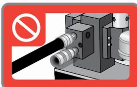
Always connect both torque wrench hoses to the pump. Do not operate with only one hose attached.
