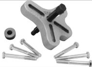
Slotted holes in puller body permit cap screws to be positioned to handle bolt-circle diameters from 1.50" - 4.63".
