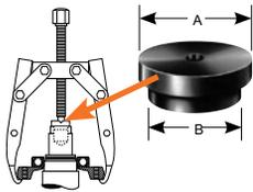
Power Team step plate adapters are necessary for pulling and installing bearings, gears, or other parts on hollow shafts or housings. Puller screw forces against step plate adapter, as shown at right. May be used with Power Team jaw-type pullers, Bi-Directional™ Pullers and shop presses.
