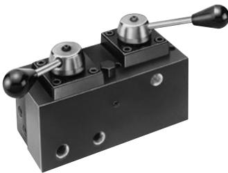
Pump-mounted, 6-position detented 5-way manual dual valve. Rated pressure to valve "A" is 10,000 psi and valve "B" is 6,000 psi. Case pressure is 500 psi max.
