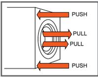
**PULLING INTERNAL BEARING RACES, RETAINER, SEALS, ETC.**
