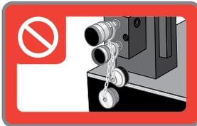
Do not operate a pump with couplers exposed or uncapped.
