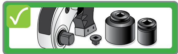
Only use high quality impact sockets and reducers with an appropriate load rating and safety factor.
