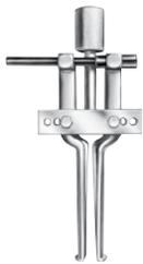
**Internal pulling attachments** have narrow jaws which extend through the center of the part to be pulled. They provide a straight pull and avoid damaging housings. Internal attachments feature adjustable jaws to fit various diameter parts.
