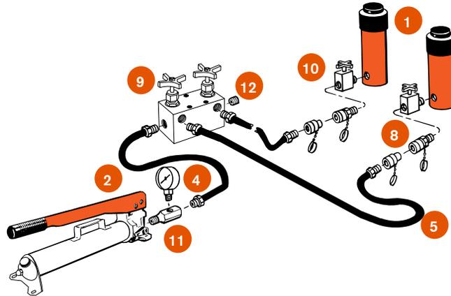
Basic double-acting system with an electric/hydraulic pump, shut-off valves, load-lowering valves and multiple double-acting cylinders.
