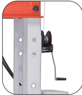
Winch provides easy positioning of press bed
