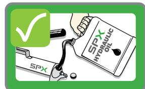
Use only high quality oil, like SPX Power Team hydraulic oil. Using the wrong fluid can lead to equipment damage and premature failure.
