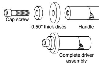
These sets have the proper-size driver for any seal, bearing or bushing installing job. Select the proper-size discs, attach to handle with cap screws and strike with hammer.
