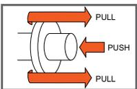
**PULLING A GEAR, BEARING, WHEEL, PULLEY, ETC., FROM A SHAFT**
