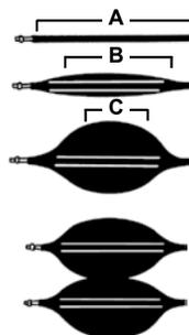
All lifting capacities mentioned in the charts are measured at the maximum effective lifting area (A). As the jack is inflated (B), this effective area decreases (C) due to the rounded shape of the jack. Lifting capacity also decreases (see performance chart).
