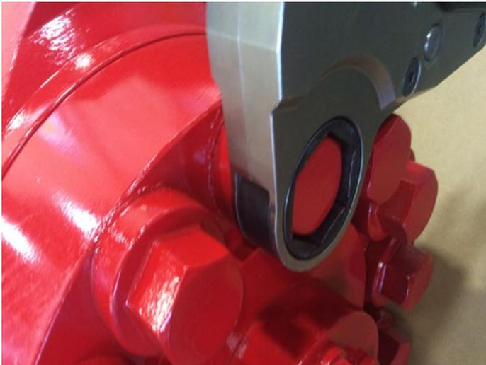
▶ The TWSL's narrow width and reduced radius design enables the tool to fit into tight areas where standard low clearance links cannot.
