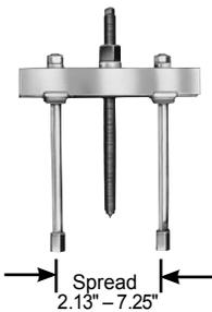
**30 Ton Capacity** can be used with 1126 and 1127 bearing pulling attachments or 680 pulley pulling attachment (two 8012 adapters are required to connect 680 to puller). Can be used with 1165 internal pulling attachment.
