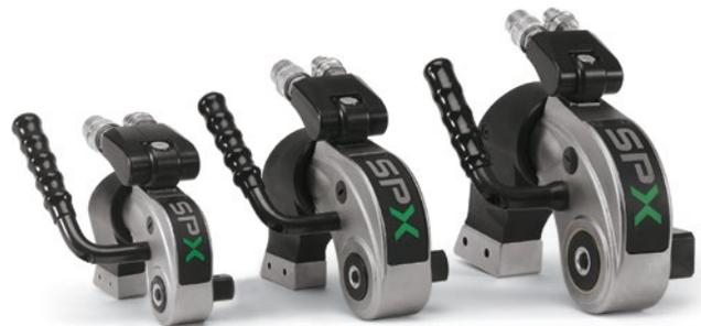
The tool's designed long-stroke mechanism imparts a minimum 30 degree nut rotation per stroke while maintaining a tight and compact nose radius. This is a clear advantage over the short stroke and back-up pawl mechanisms of light alloy competitive models. Fewer parts and reduced torsion in operation equals reduced wear, maintenance and associated costs.
