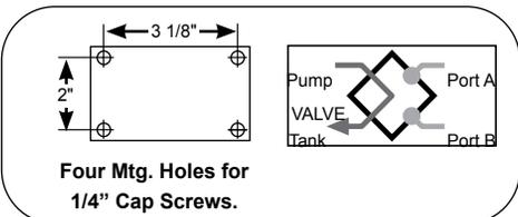
**4-WAY / 3-POSITION (TANDEM CENTER) SOLENOID VALVE WITH POSI-CHECK®**
