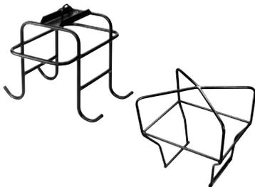
Safeguards pump, gas engine and valves on the job site. Horizontal bars provide convenient hand holds for carrying pump, a pick-up point permits lifting unit with an overhead crane or other device. Standard equipment on PG1203 and PG1204. Can be ordered as an option with any other gas, air, or electrically driven hydraulic pump equipped with a 5-gallon reservoir.
