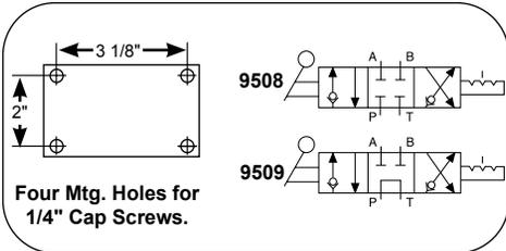
**4-WAY / 3-POSITION (CLOSED CENTER) AND (TANDEM CENTER) MANUAL VALVES WITH POSI-CHECK®**
