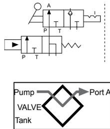
**Applications:** Manual operation for load lifting and holding with single-acting cylinders; automatic "dump" for operating hydraulic tools.
