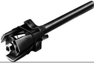
This installer adjusts to fit bearing cups from 3.63" - 6.50" O.D. It replaces over two dozen plates and drivers. Simply adjust the jaws to fit the cup I.D., lock the jaws, slip the new cup on and drive it home with a hammer.
