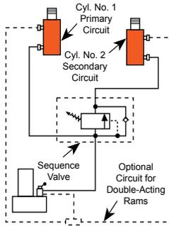
**Application:** Used when one cylinder in a multi-cylinder application must advance before any other.
