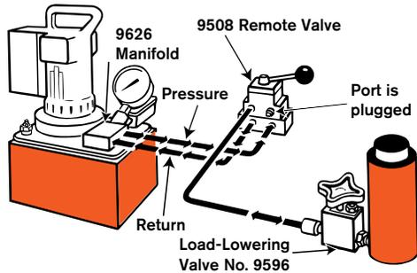
Double-acting cylinders controlled by a remote-mounted valve.
