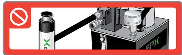
Do not use pumps designed for torque wrenches or tensioners for lifting.
