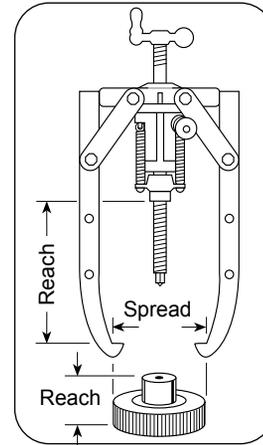
**▲ CAUTION:** Always use a 3-jaw puller where clearance permits in order to provide a more stable setup and a more even pulling force.
