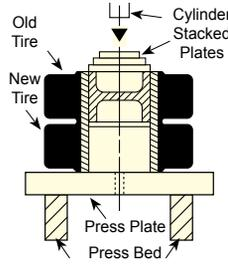
Now an easy way to press solid rubber tires. The TPP200 uses plates instead of combination rings to press a rim from an old tire into a new one. P They can be used on any Power Team press with 55 ton capacity or more.
