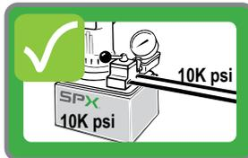
Recognize system pressures. Do not use a 10,000 PSI pump on a system with 3,000 PSI components (hoses, fittings, valves, tools, etc.).
