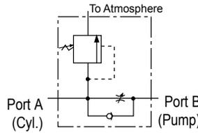
**Application:** Precision metering for controlled cylinder piston return.
