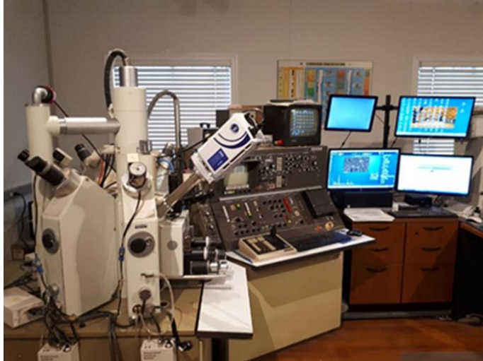
Figure 15 Photo of the JEOL JXA-733 electron microprobe housed at the laboratory of Renaud Geological Consulting Ltd., London, ON. This is the location where petrographic and ore mineral characterization occurred.
