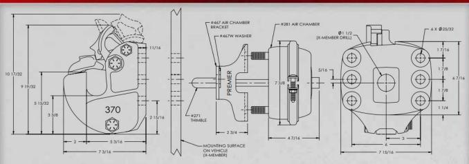
Pushrod length is 4 in. [102 mm] plus thickness of mounting structure for standard installations as illustrated.
