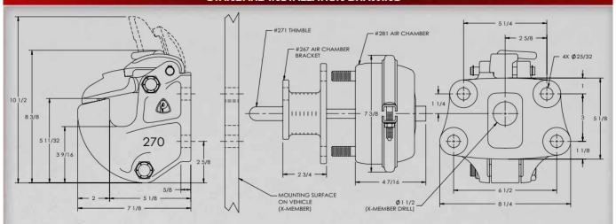
Pushrod length should be 3 5/8 in. (92 mm) plus thickness of mounting structure for standard installations as illustrated.
