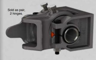
Accepts 3 in. (76 mm) standard channel or square tubing. 448 Rubber Bushings standard, 448A Poly optional (440A)
