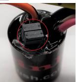
Connect the module to the 8-way throttle body connector of the engine wiring harness and to the new throttle body. There will be a "click" when the connection is secure. If you don't hear/feel the click, check that the center portion (purple or grey) that covers/aligns the pins is fully seated.
