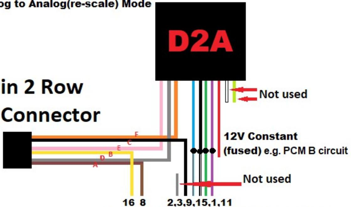
**Factory throttle Body Wiring From TAC Module C1**
