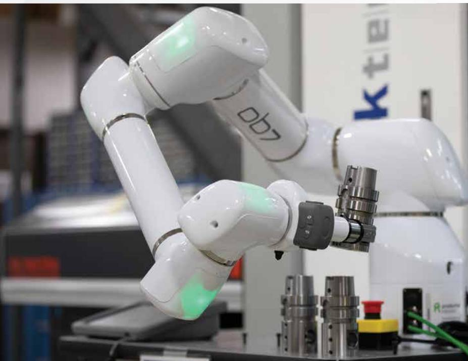
There are several collaborative robots out there, but OB7's 7 axes allow us to place the robot next to the machine door rather than in front of it, freeing up space for our machine operators. The ease of setting up OB7 has also made us profitable in our job shop environment from day one.
