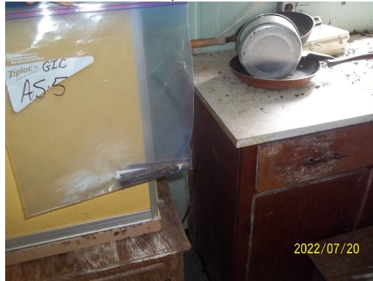
Photo 16: View of bulk material sample GIC AS-5, countertop mastic, cabin interior.
