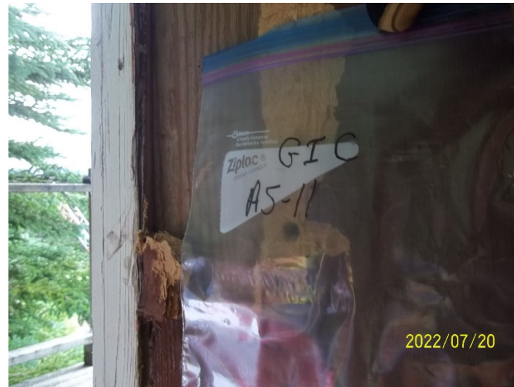
Photo 22: View of bulk material sample GIC AS-11, caulking, cabin exterior.
