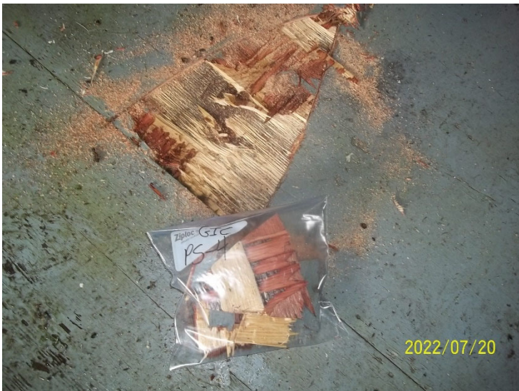
Photo 27: View of paint sample GIC PS-4, floor, cabin interior.
