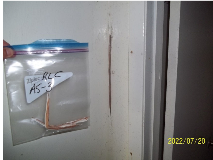
Photo 10: View of bulk material sample RLC AS-3, caulking, cabin interior.
