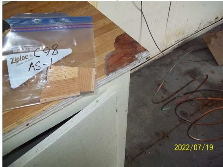
Photo 12: View of bulk material sample C98 AS-1, countertop mastic, cabin interior.
