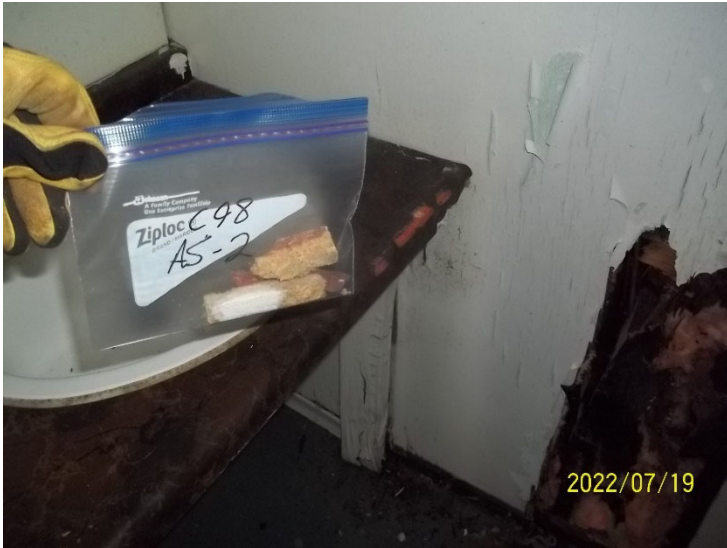
Photo 13: View of bulk material sample C98 AS-2, countertop mastic, cabin interior.
