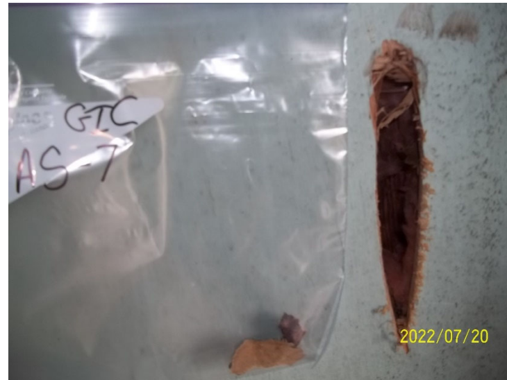
Photo 18: View of bulk material sample GIC AS-7, fibreglass and tar paper, cabin interior.
