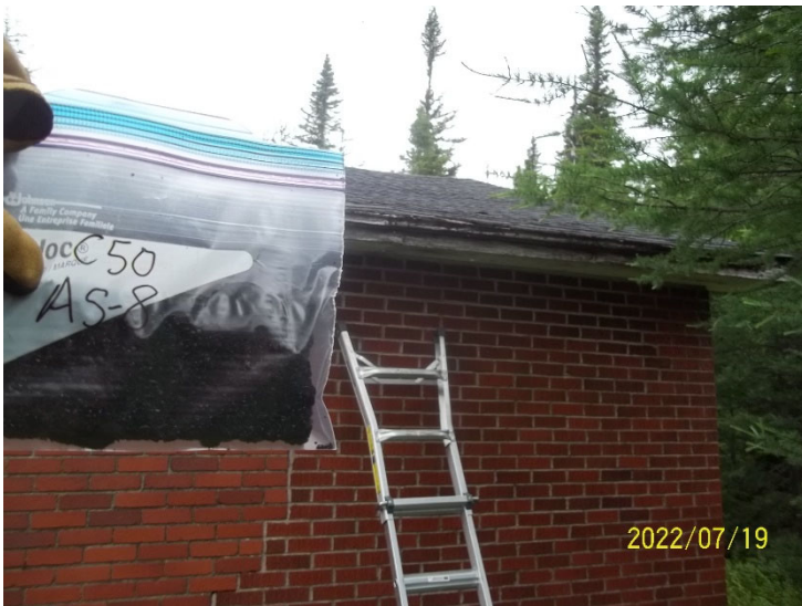
Photo 19: View of bulk material sample C50 AS-8, shingle and tar paper, cabin exterior.
