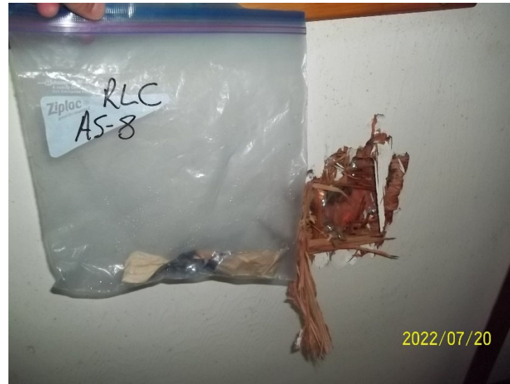
Photo 14: View of bulk material sample RLC AS-8, foil paper, cabin exterior.
