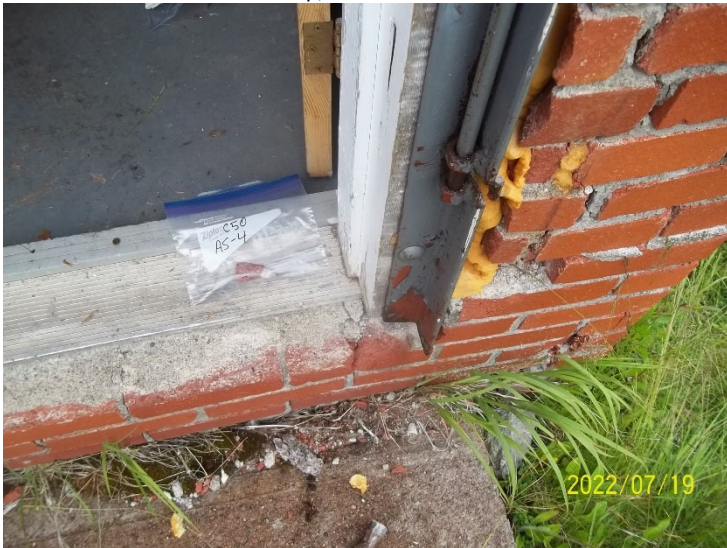
Photo 15: View of bulk material sample C50 AS-4, brick and mortar, cabin exterior.
