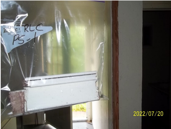
Photo 17: View of paint sample RLC PS-1, wall, cabin interior.
