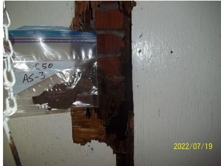
Photo 14: View of bulk material sample C50 AS-3, particle board, cabin interior.
