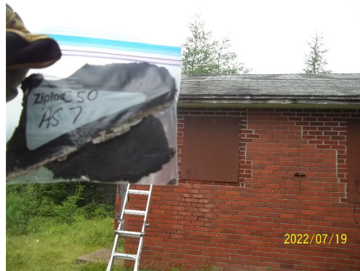
Photo 18: View of bulk material sample C50 AS-7, shingle and tar paper, cabin exterior.
