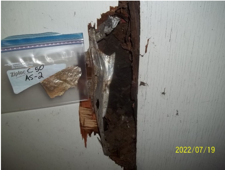
Photo 13: View of bulk material sample C50 AS-2, foil wrap, cabin interior.
