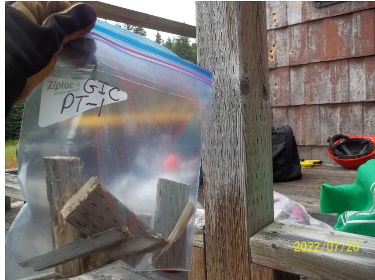
Photo 30: View of treated wood sample GIC PT-1, cabin exterior.
