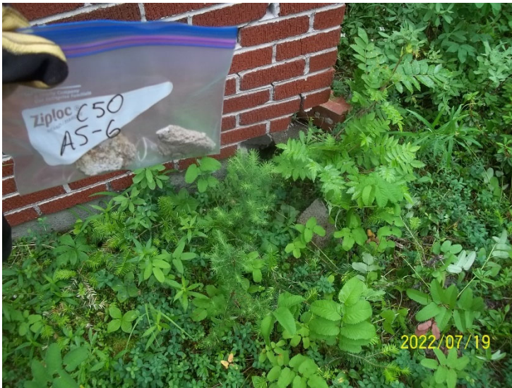
Photo 17: View of bulk material sample C50 AS-6, cinder block and mortar, cabin exterior.
