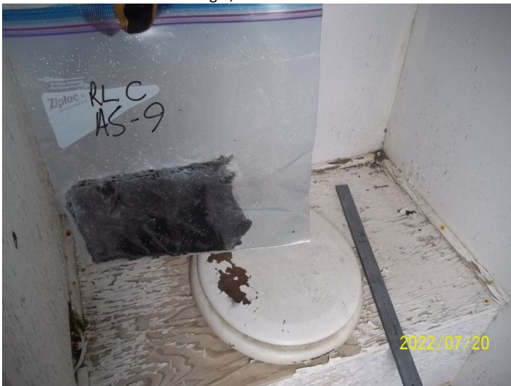
Photo 15: View of bulk material sample RLC AS-9, shingle, outhouse exterior.
