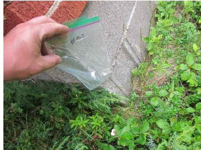
Photo 20: View of bulk material sample NP-AS7, concrete block, cabin exterior.
