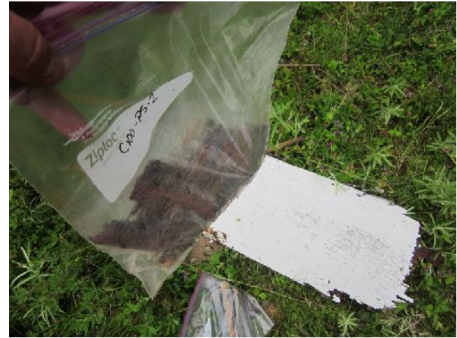
Photo 18: View of paint sample C100-PS-2, white, cabin interior.
