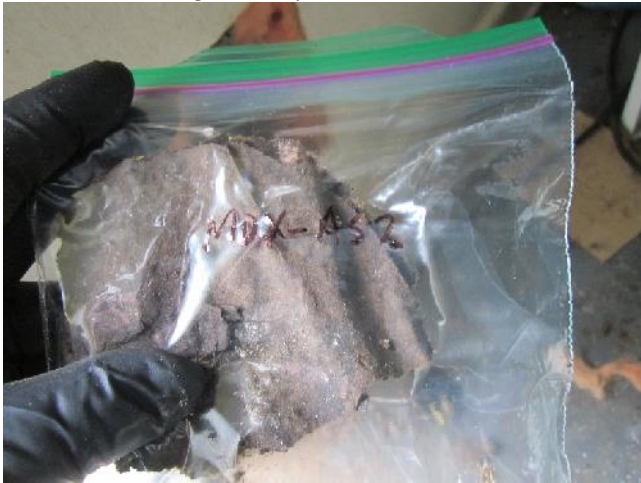
Photo 15: View of bulk material sample MDX-AS2, black pressboard and tar paper, Room 1.
