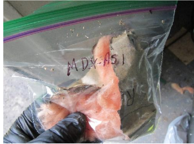
Photo 14: View of bulk material sample MDX-AS1, black paper on fibreglass insulation, Room 1.
