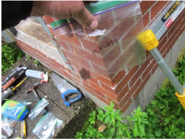
Photo 17: View of bulk material sample MDX-AS4, red brick, cabin exterior.
