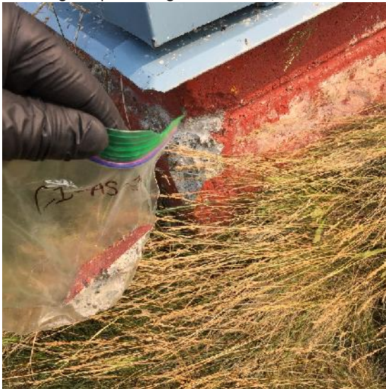
Photo 19: View of bulk material sample C1-AS-3, concrete, cabin exterior.
