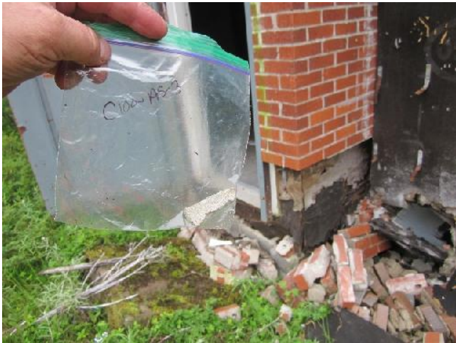
Photo 15: View of bulk material sample C100-AS-3, grey mortar, cabin exterior.
