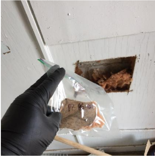
Photo 17: View of bulk material sample PP-AS-1, black paper backing and pink fibreglass insulation, cabin interior.
