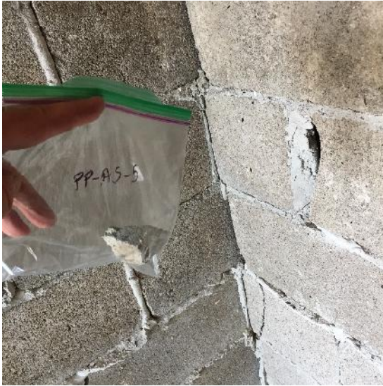
Photo 21: View of bulk material sample PP-AS-5, concrete block and mortar, cabin exterior.
