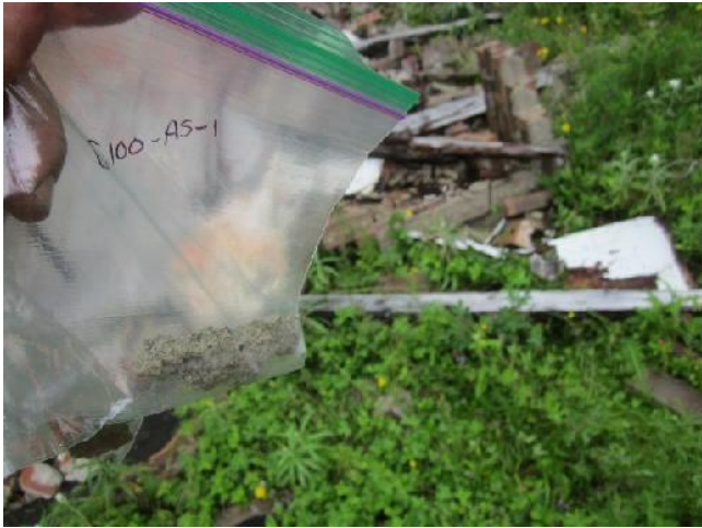
Photo 13: View of bulk material sample C100-AS-1, grey mortar, cabin exterior.
