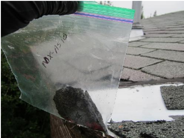
Photo 23: View of bulk material sample MDX-AS10, black shingle and tar, cabin exterior.
