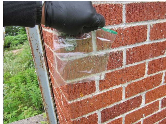
Photo 16: View of bulk material sample HG-AS4, grey mortar, cabin exterior.
