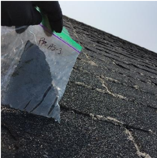
Photo 19: View of bulk material sample PP-AS-3, black shingle, cabin exterior. 2.2 % Crysotile Asbestos
