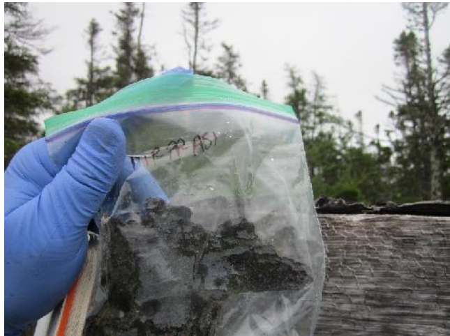
Photo 24: View of bulk material sample MP-PP-AS1, black shingle and tar, cabin exterior.
