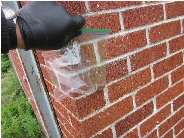
Photo 17: View of bulk material sample HG-AS5, red brick, cabin exterior.
