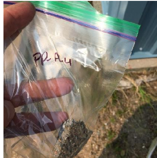
Photo 20: View of bulk material sample PP-AS-4, concrete, cabin exterior.
