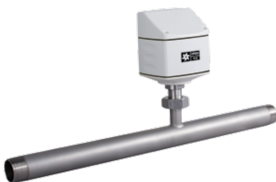
OS 421: Shortened inlet section! Recommended inlet section length is: l = 15 \times \text{inner pipe diameter}
