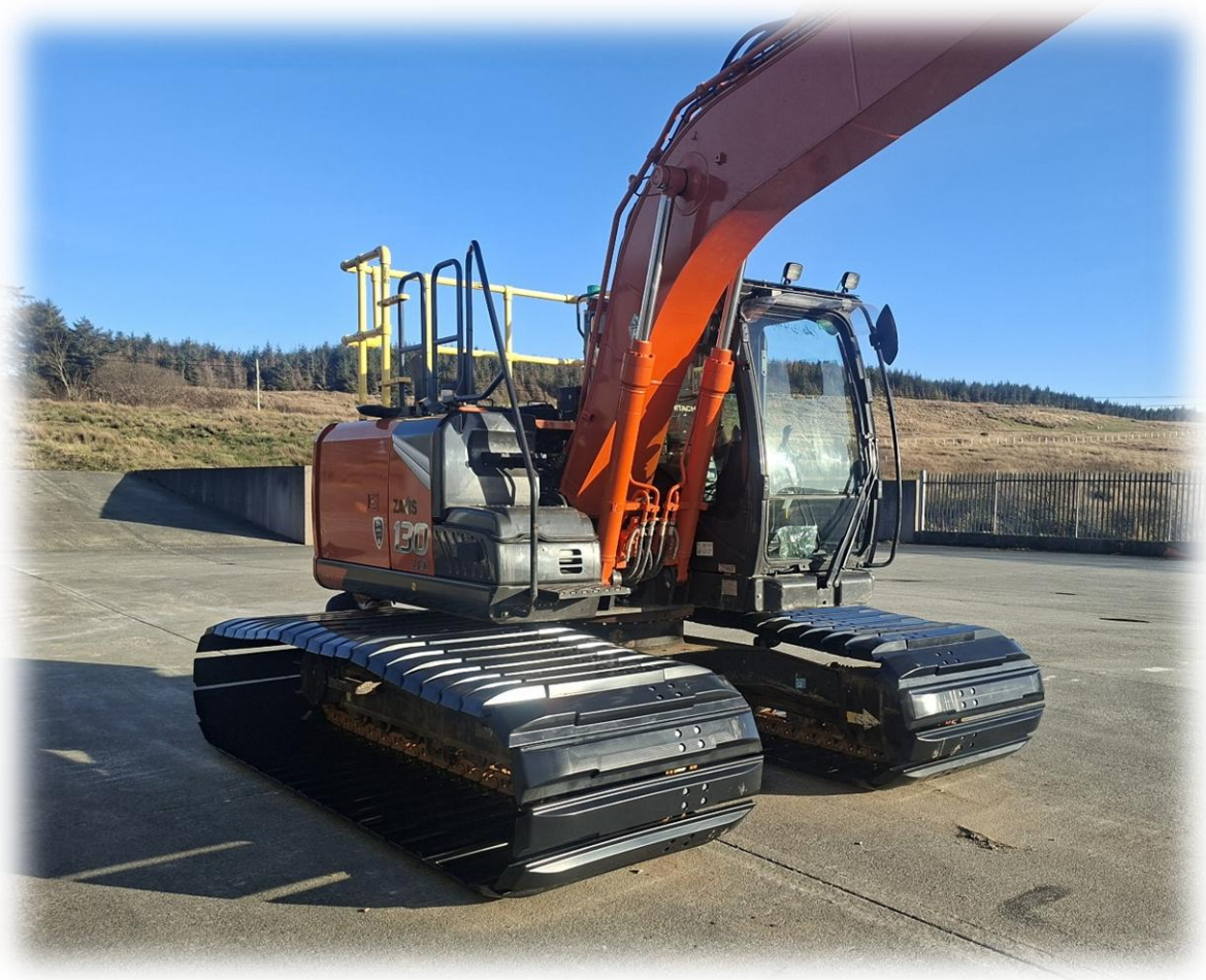
Hitachi 130 LCN-7 with track pad offset 470-830mm
