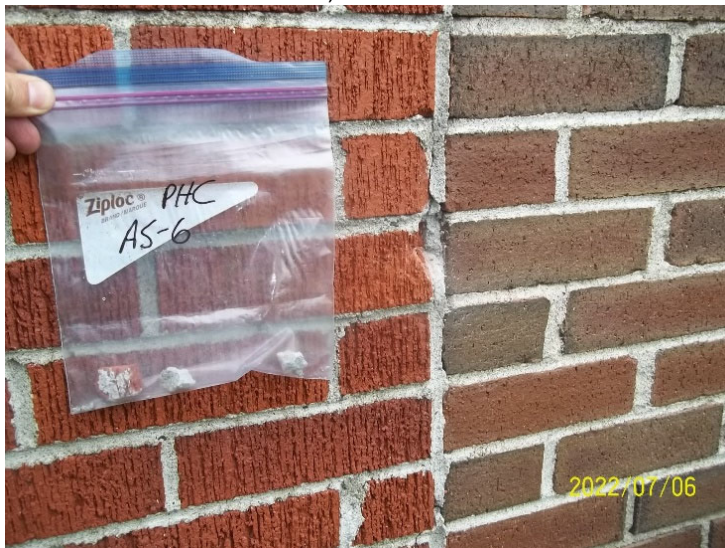
Photo 15: View of bulk material sample PHC AS-6, brick and mortar, cabin exterior.
