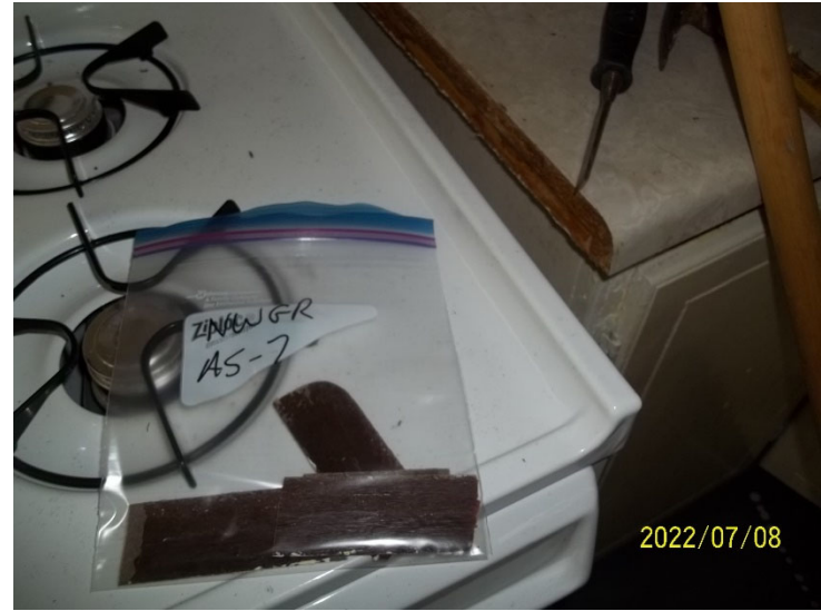
Photo 18: View of bulk material sample NWGR AS-7, countertop mastic, cabin interior.
