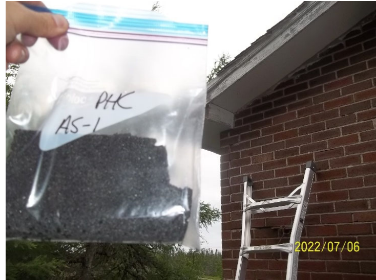
Photo 10: View of bulk material sample PHC AS-1, shingle, cabin exterior.
