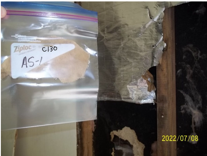
Photo 15: View of bulk material sample C130 AS-1, foil/tar paper backing on fibreglass insulation, cabin interior.
