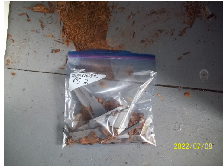
Photo 22: View of paint sample NWGR PS-2, floor, cabin interior.
