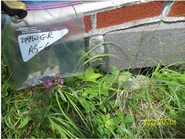
Photo 17: View of bulk material sample NWGR AS-6, cinder block and mortar, cabin exterior.
