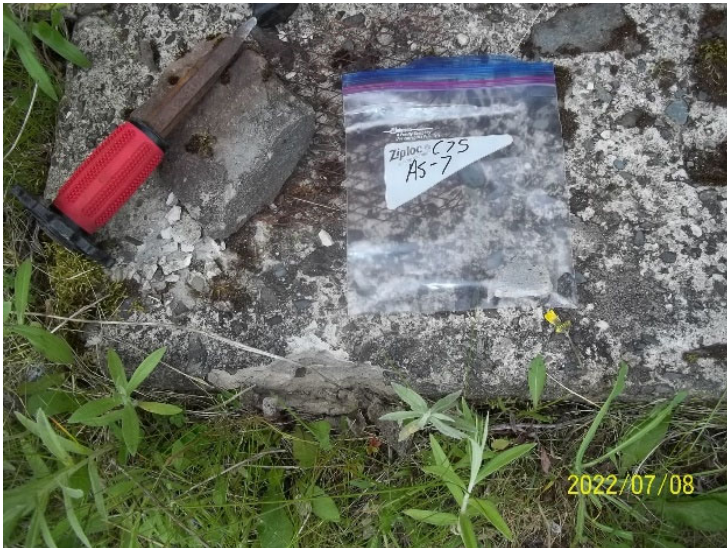
Photo 19: View of bulk material sample C75 AS-7, concrete, cabin exterior.
