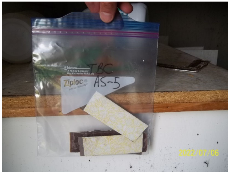
Photo 19: View of bulk material sample TBC AS-7, countertop mastic, cabin interior. Note: sample was mislabeled.
