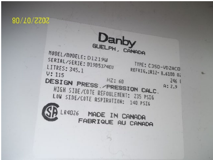
Photo 31: View of label inside freezer indicating refrigerant R12.
